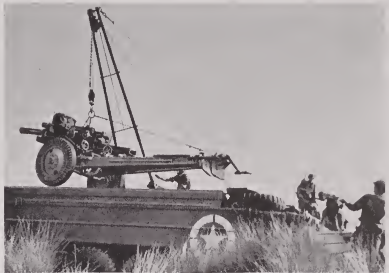
FIGURE 20. Unloading 105-mm howitzer from DUKW by means of A-frame on another DUKW.
